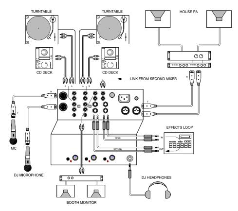
**DJ Microphone and Headphones:** The DJ plugs in the preferred headphones and microphone. A second mic for the MC may also be required. The console cue system works with the headphones to let the DJ cue tracks and preview the mix before going live.
